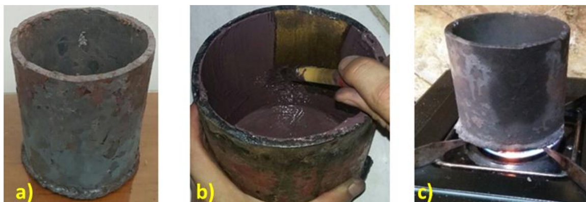
Figure 1. Steel crucible: a)Prior to coating; b)Coating, c)Heating of steel crucible
