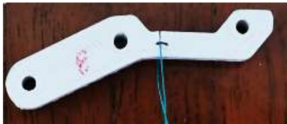
Figure 14. Measuring crack depth with a thread
