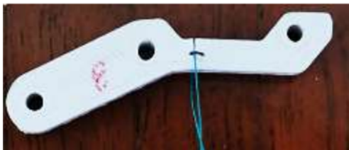
Figure 14. Measuring crack depth with a thread
