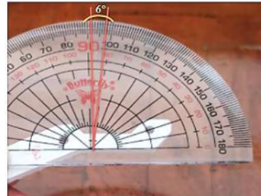
Figure 9. Crack angle measurement technique
