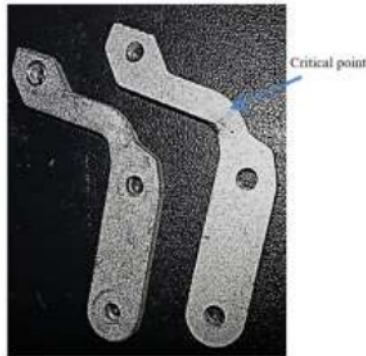
Figure 13. Aluminium gripper test results
