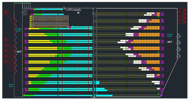
Figure 4. The application of class-based storage method shelves (The colors yellow and orange indicate class A; The colors green and purple indicate class B)
