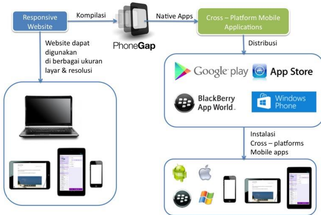
Gambar 1.3. Block Diagram Sistem Responsive Website dan Cross-Platform Mobile Applications (Sumber: Olahan Peneliti (2014) )
