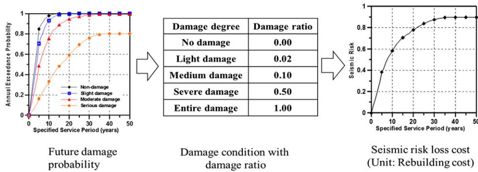
Figure 6. Method used to obtain the earthquake maintenance cost ( $C_{ME}$ ).
