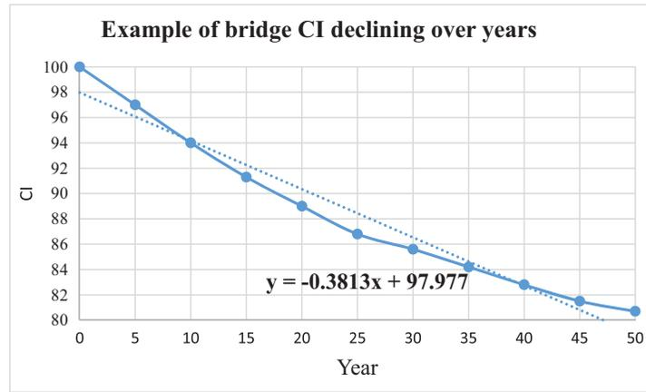
Figure 3. Decline in CI over time (beam/girder type bridges).
