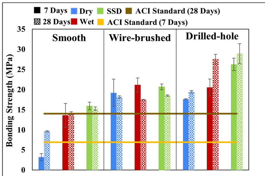
**Figure 6.** Slant shear test result.
