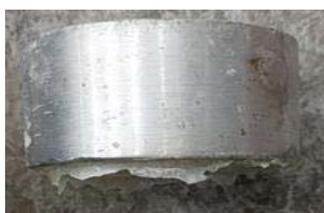
Figure 9. Epoxy failure at steel disk.
