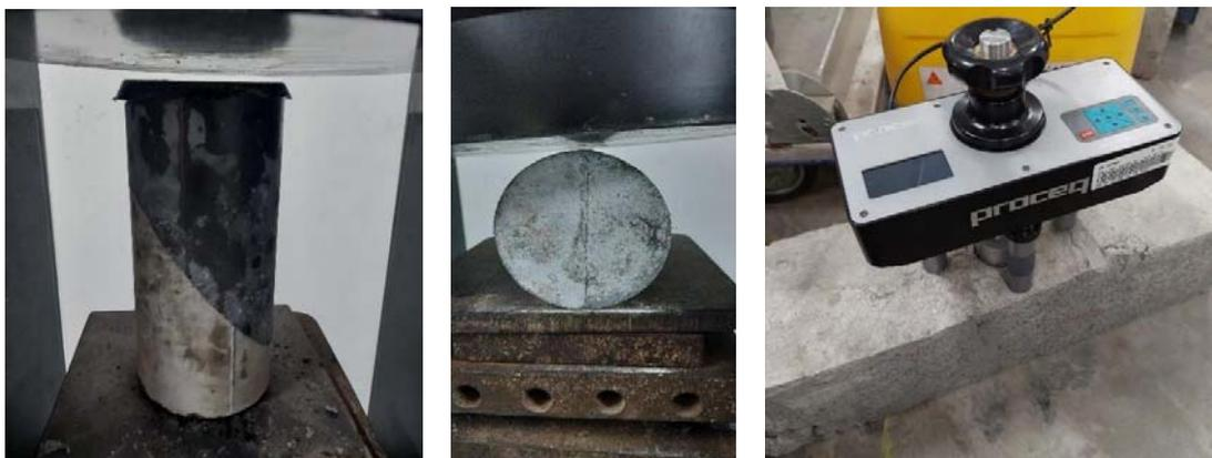
*Slant-shear*                      *Splitting Tensile*                      *Pull-off*
