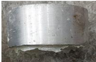
Figure 9. Epoxy failure at steel disk.
