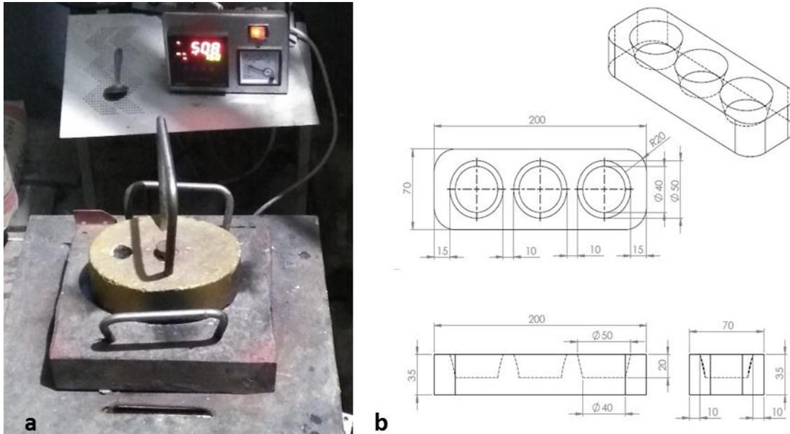
Figure 2. a) Electrical resistance furnace, b) The die
