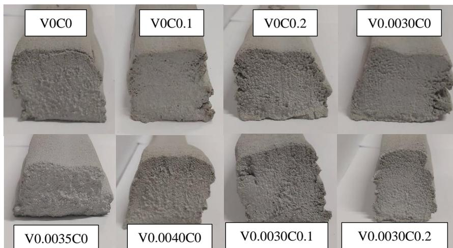
**Figure 9.** Cross sections of the printed mix designs.
