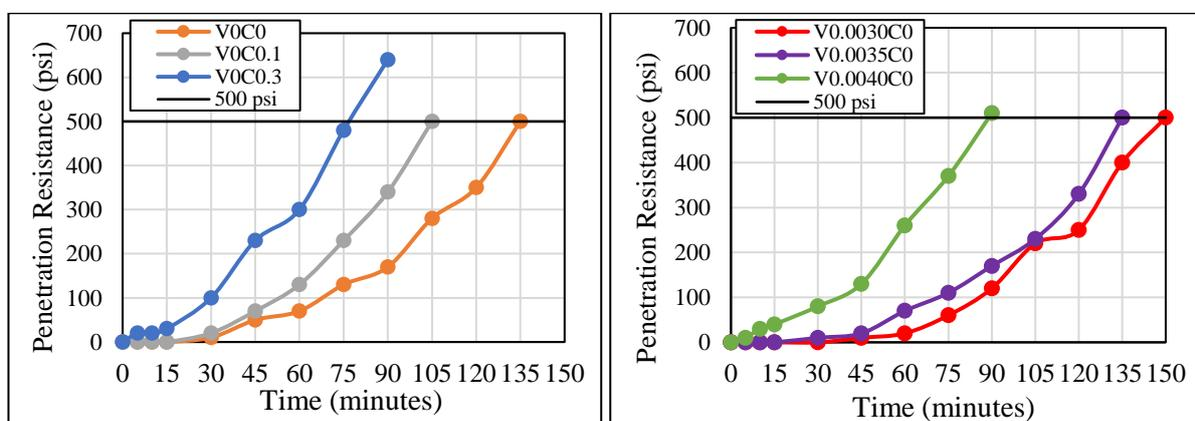
Figure 4. Initial setting time of mixture with the variation of (a) CaCO<sub>3</sub> and (b) VMA dosage.
