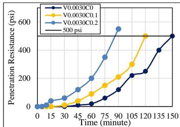
**Figure 5.** Initial setting time of combined CaCO<sub>3</sub> and VMA.
