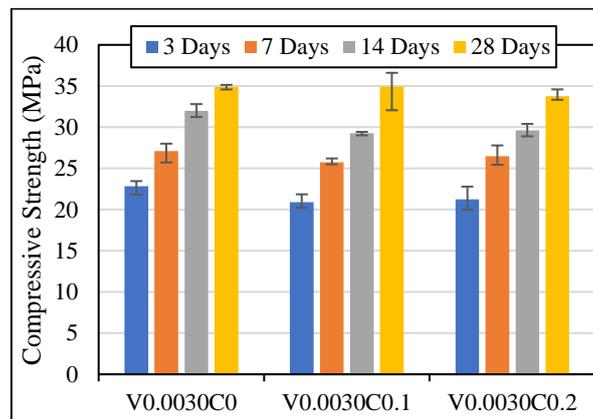
**Figure 7.** Compressive strength of combined CaCO<sub>3</sub> and VMA.
