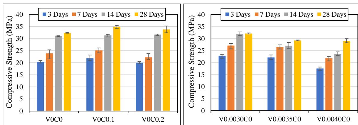
**Figure 6.** Compressive strength for the mixture with the variation of (a) CaCO<sub>3</sub> and (b) VMA dosage.
