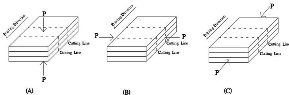
**Figure 2.** Compressive test directions.
