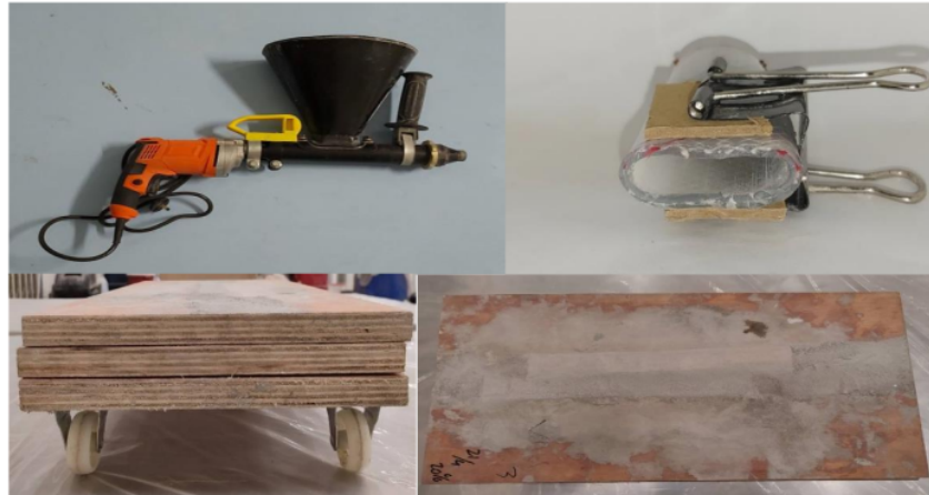
Figure 1. A mortar extruder, nozzle, and printing bed are used for mortar extrusion.
