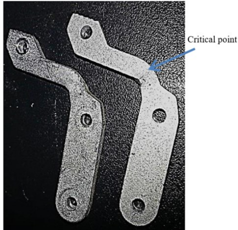
FIGURE 11. Aluminium gripper test results
