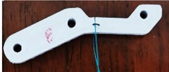
FIGURE 12. Measuring crack depth with a thread
