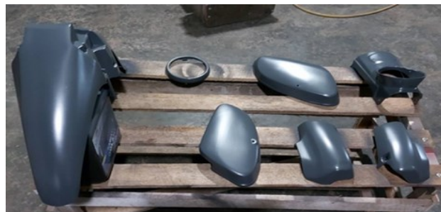
FIGURE 9. The finishing and painting of the C-70 motorcycle
