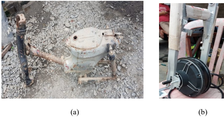
FIGURE 1. The pressed steel frame used in the C-70 motorcycle (a), BLDC motor fitting on the swing arm (b)
