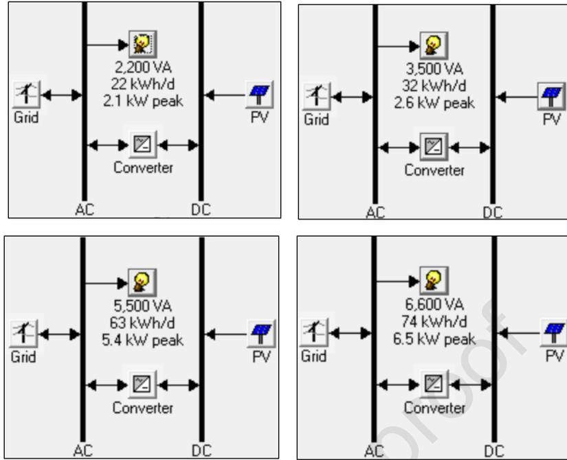
Figure 4. HOMER system configurations for residential households with 2,200 VA and 3,500 VA (top left to right), households with 5,500 VA and 6,600 VA (down left to right) electricity contracts.
