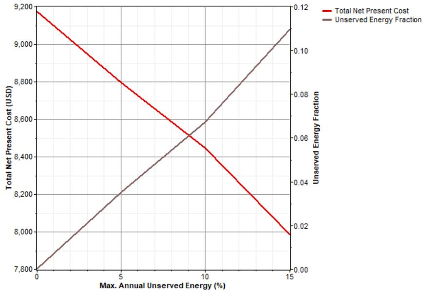
26 Figure 13. Sensitivity result of total NPC versus unserved energy fraction in a 2,200 VA household with 100%-
