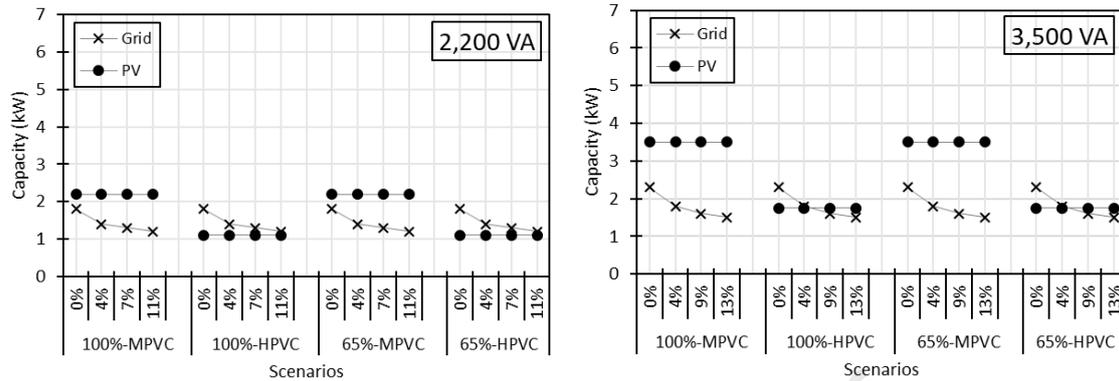
Figure 11. System capacity across all unserved energies for 2,200 VA (left) and 3,500 VA (right)
