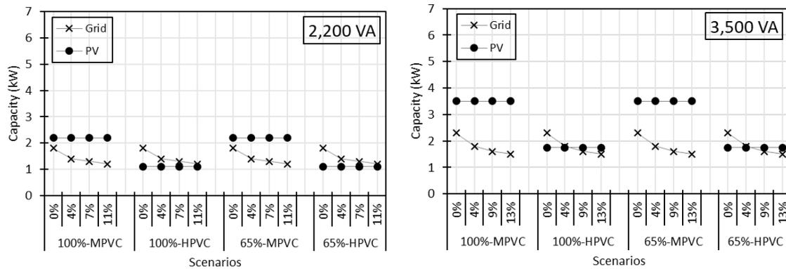
Figure 11. System capacity across all unserved energies for 2,200 VA (left) and 3,500 VA (right)
