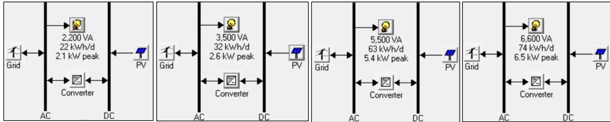
Figure 4. (Left to Right) System configurations for residential household with 2,200 VA, 3,500 VA, 5,500 VA, and 6,600 VA electricity contract in HOMER.
