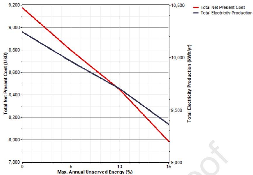
Figure 15. Sensitivity result of total NPC versus total electricity production in a 2,200 VA household with 100%-MPVC.
