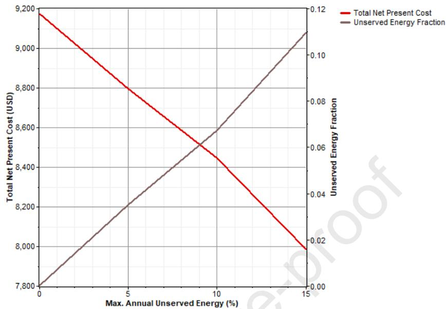
Figure 13. Sensitivity result of total NPC versus unserved energy fraction in a 2,200 VA household with 100%-MPVC.
