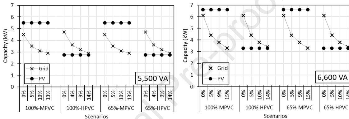
Figure 12. System capacity across all unserved energies for 5,500 VA (left) and 6,600 VA (right)
