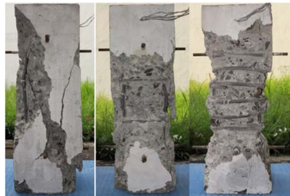
Fig. 19. Specimens CS-01, CS-02a, and CS-03a after the accomplishment of the tests
