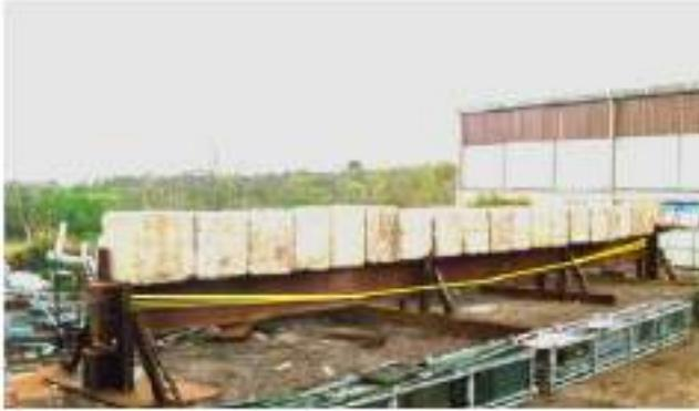
**Gambar 15.36** Uji Pembebanan Balok Baja Prategang Tendon Poligon
