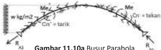
**Gambar 11.10a** Busur Parabola terhadap Beban Lateral
