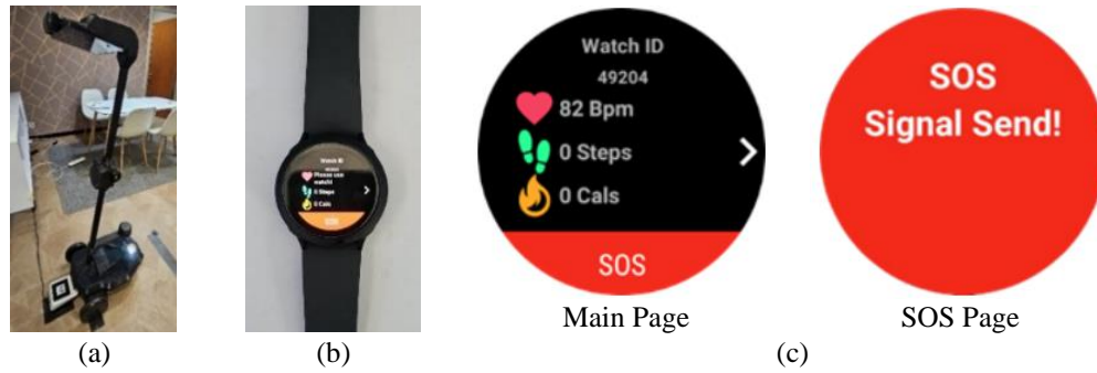
Figure 2. The robot and the mobile application for the elder: (a) the telepresence robot, (b) the smartwatch, and (c) mobile application
