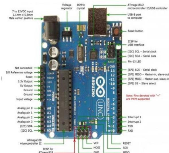
Gambar 2. Board Arduino Atmega328
