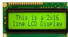
Gambar 4. LCD 2x16
