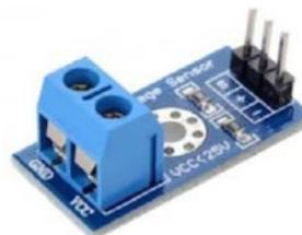
Gambar 3. Sensor Tegangan DC
