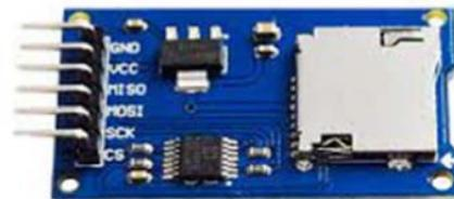
Gambar 8. Modul Micro SD Card
