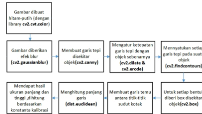
Figure 6. The process of object sizes measurements
