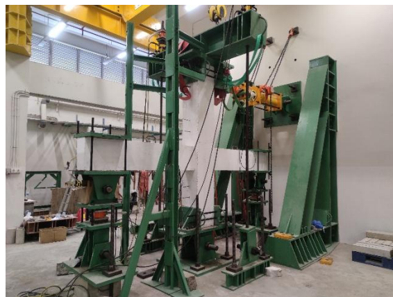
Figure 2. Overall Test Setup of the RC Beam-column Joint Specimen
