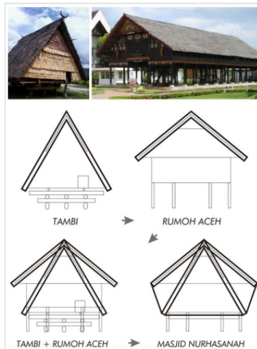
Figure 7. Top: Tambi house and Rumoh Aceh (Kevin 2020; Wikipedia 2022) Bottom: Roof geometry concept
