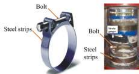
Figure 1. Column Specimen Retrofitting with Steel Clamp.
