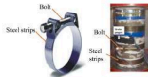
Figure 1. Column Specimen Retrofitting with Steel Clamp.
