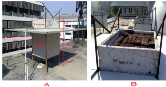
Source: (Mintorogo, 2010) Figure 4: A. The model, B. Covered model with Pakis-stem Blocks
