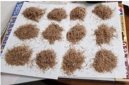
Figure 3 A mixture of bagasse and rice husk was placed on top of PLA sheet to make a sandwich
