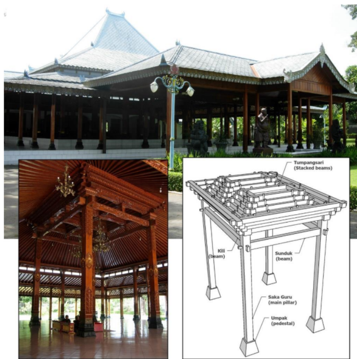
Fig. 1: Rong-rongan , the core structure of the joglo building.
