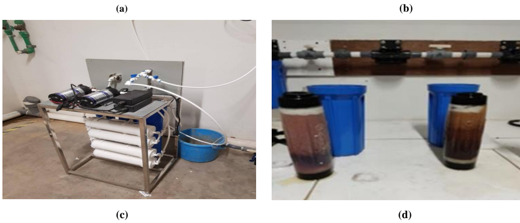
Figure 4. Water treatment equipment assembly. Preparation for filter module, reverse osmosis, ion exchanger in filter module and obtaining brackish water sample
