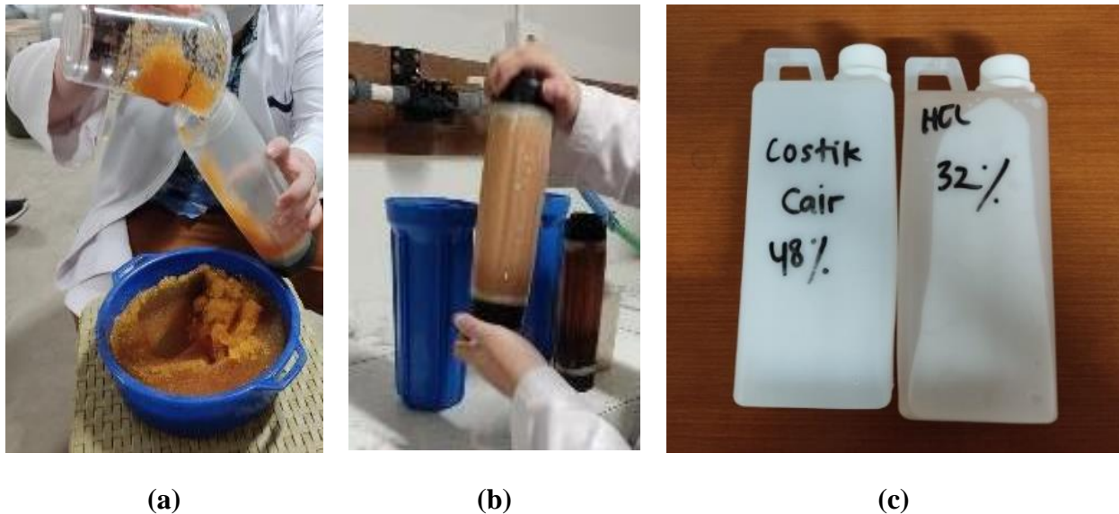
Figure 3. Material for Ion Exchanger. Anion and Kation Exchanger Resin
