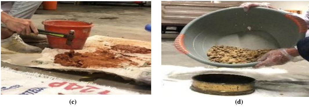
Figure 5. Filter media pre treatment phase. Washing, drying, crushing and screening
