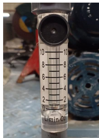
Gambar 4. Flow meter gas
