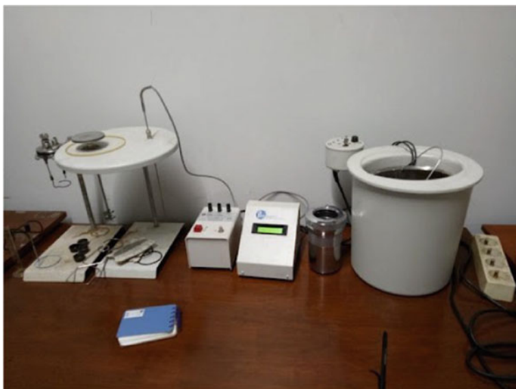
Fig. 14.7 Oxygen bomb calorimeter
