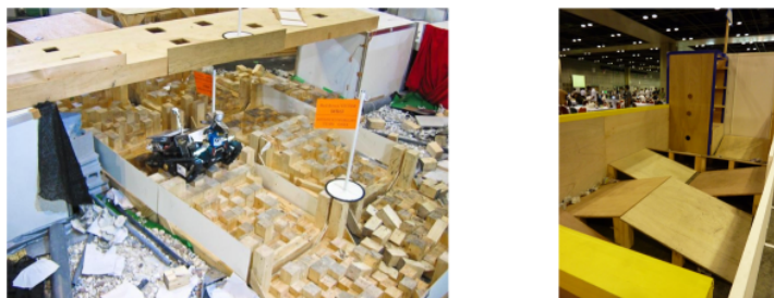
Fig. 1.3 Elements of a typical robot rescue arena
