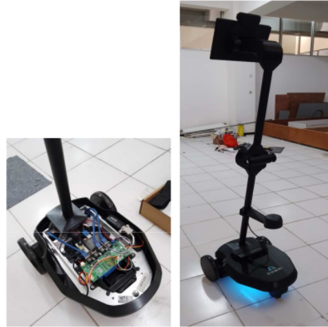
Fig. 3. The Ohmni Robot is opened and equipped with a LIDAR sensor
