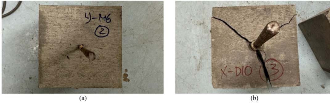
Figure 9. Failure Modes of the Specimens; (a) Pull-out (slip) Failure and (b) Splitting (split) Failure
