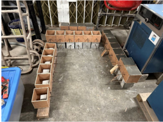
Figure 5. Small Cubes Placed in the Formwork (left) and Grouting Material used as Filler (right)
