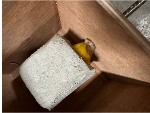
Figure 6. Protection for the Steel Reinforcement using Combination of Clear Tape, PVC Pipe (covered), and Clay
