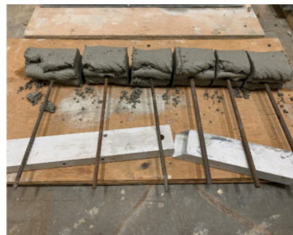
Figure 4. Printed Small Cubes
