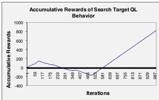
Figure 14. Accumulated rewards which are accepted by robot for QL search target behavior
