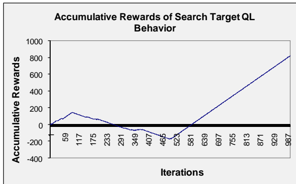
Figure 14. Accumulated rewards which are accepted by robot for QL search target behavior
