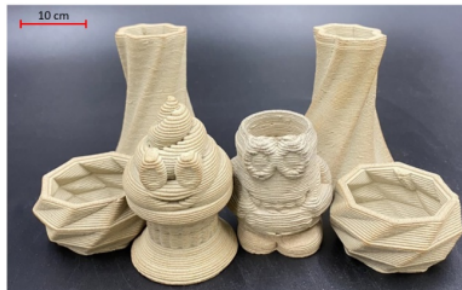
Fig. 5. Printed parts of the recycle oyster shell and clay
