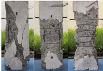
Fig. 19. Specimens CS-01, CS-02a, and CS-03a after the accomplishment of the tests
