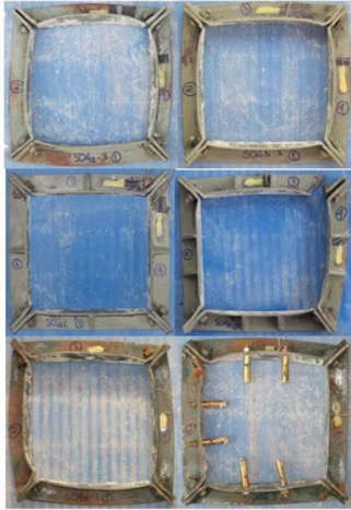
Fig. 22. Steel collars of Specimens S-04a, S-04b, S-04c, S-04d, S-04e, and S-04f after accomplishment of the tests
