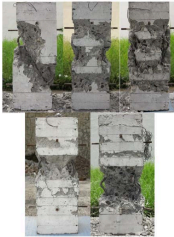
Fig. 20. Specimens S-01, S-02, S-03, S-04, and S-05 after the accomplishment of the tests
